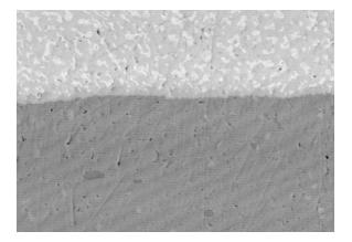
60 Seconds Above Liquidus Intermetallic layer thickness of 0.50 microns
