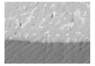
120 Seconds Above Liquidus Intermetallic layer thickness of 1.25 microns
