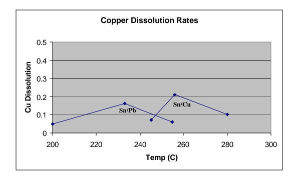
As an aside, relatively rapid intermetallic growth can occur over time when exposed to constant high temperature. (Although this will also occur even room temperature, these growth rates are generally so low as to not affect a device during its field service). As the graphs below demonstrate, alloys that already contain a percentage of the base metal generally better inhibit intermetallic growth over long periods of time when exposed to
