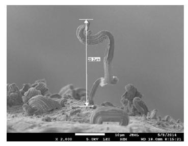
FIGURE 1. The largest whisker grown by the top performing alloy, Sn0.6Ag0.6Cu3Bi.
