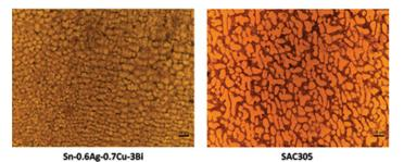
FIGURE 2. Grain structures of low-whiskering SAC-Bi alloy and highwhiskering SAC305.
