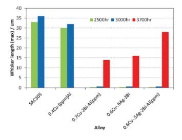
FIGURE 3. Maximum observed whisker size after storage at 60°C and 85%RH.
