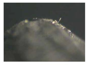
FIGURE 3. Whisker growth on outside, or tension side of bend.
