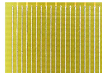
FIGURE 7. Paste 16 Post T Shock/No defects
