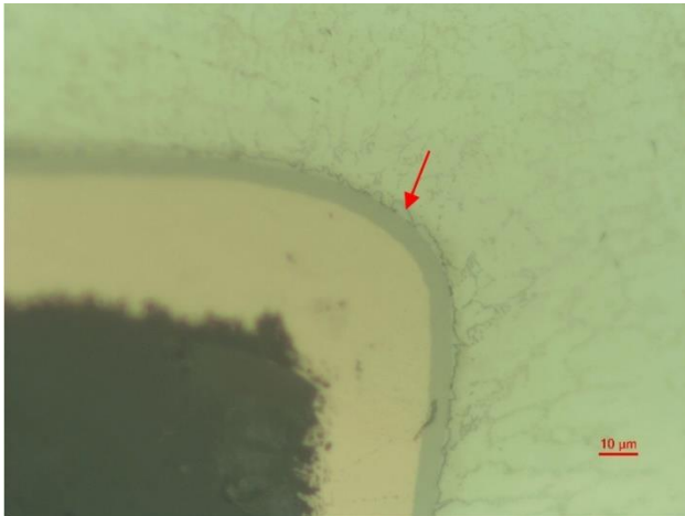
Figure 9. R1 PTH component assembled with Sn42/Bi57/Ag1 paste reworked with SAC flux cored wire
