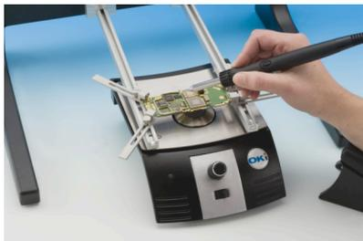
**OK International has introduced a focus pre-heater for enhanced process control during lead-free hand assembly and rework. The PCT-100 uses convection air heating, to maximise responsiveness and thereby avoid temperature overshoot that can damage**
