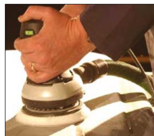
Figure 3 On-tool extraction – hand sander
