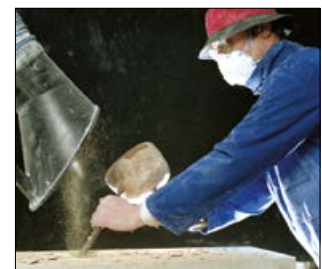
Figure 4 Fixed capturing hood
