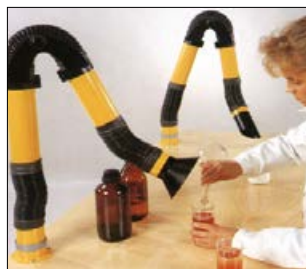
Figure 5 Moveable capturing hood
