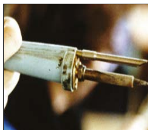
Figure 2 On-tool extraction – soldering iron
