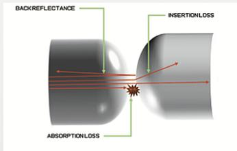
Contaminated end faces can cause back reflectance, absorption loss and insertion loss
