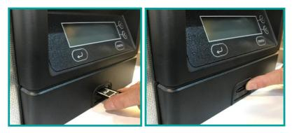
The memory card can be connected to a PC, using this memory to USB card reader to give a permanent electronic record of the cleaning parameters of the cycle.
