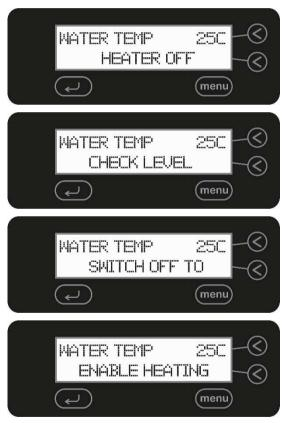
To continue using your Qi-Series ultrasonic bath, refill with liquid up to the level sensor, switch the unit off and on again.
