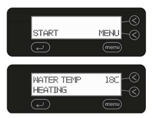
When the water temperature is at or above the temperature set, the message "Temp OK" will display.
