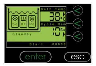
When the heaters are in operation, the symbol above Ht will oscillate showing the heaters are in operation.
