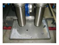
**Step 2** - Turn both valves 90 degrees to the "off / "closed" position to isolate the tank fluid:
