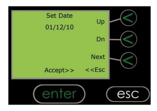
The **Neon Series** is factory pre-set with the correct date. If the date should be incorrect, use this screen to amend it.
