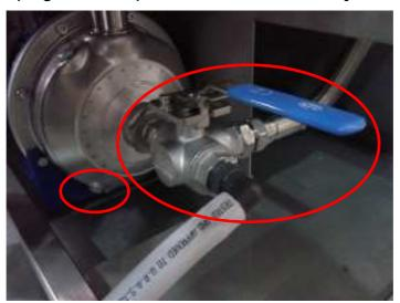
**Step 1** - Ensure that the drain (on rear of unit) is connected to a suitable drain outlet or container.
