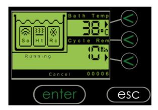
The **Neon Series** cycle will now begin, indicated by the 'Running' message on the display. The ultrasonic cycle will run for the programmed time and any re-circulation will also run once at the cycle start point, and once at the end of the cycle.
