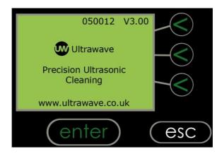
While this screen is displayed, the buttons are inoperative. This is normal as the **Neon Series** is running through its start-up routine and checking all internal systems are working correctly.
