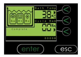
The user must acknowledge the complete cycle, by pressing the enter button, before the screen will return to the start ready for another cycle to be started.
