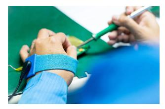
Walking alone can create static electricity and ESD matting can help to disperse this electricity through electrically conductive carbon fibres woven throughout. Consequently, the ESD flows at a slower rate across the surface of the mat which in turn neutralises it. There is also matting available which is appropriate to use on workbenches, trolleys and other surfaces.
