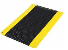
Antistatic mats help to protect static sensitive components from electrostatic discharge. They are engineered to drain static discharge from items placed on their surface. They also serve to protect the surface of the ESD sensitive devices from wear and tear by slowing down the flow of static charge, and moving the charge into the grounded mat, away from the components.
