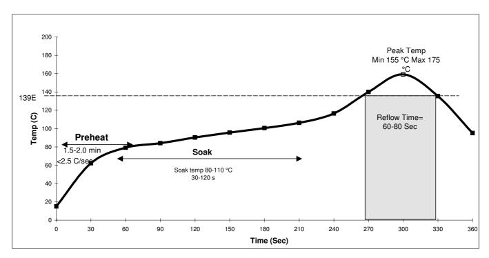
**Preheat Zone**- The preheat zone, is also referred to as the ramp zone, and is used to elevate the temperature of the PCB to the desired soak temperature. In the preheat zone the temperature of the PCB is constantly rising, at a rate that should not exceed 2.5 C/sec. The oven's preheat zone should normally occupy 25-33% of the total heated tunnel length.
