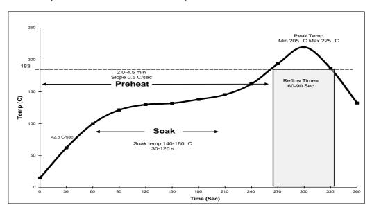
**Preheat Zone**- The preheat zone, is also referred to as the ramp zone, and is used to elevate the temperature of the PCB to the desired soak temperature. In the preheat zone the temperature of the PCB is constantly rising, at a rate that should not exceed 2.5 C/sec. The oven's preheat zone should normally occupy 25-33% of the total heated tunnel length.
